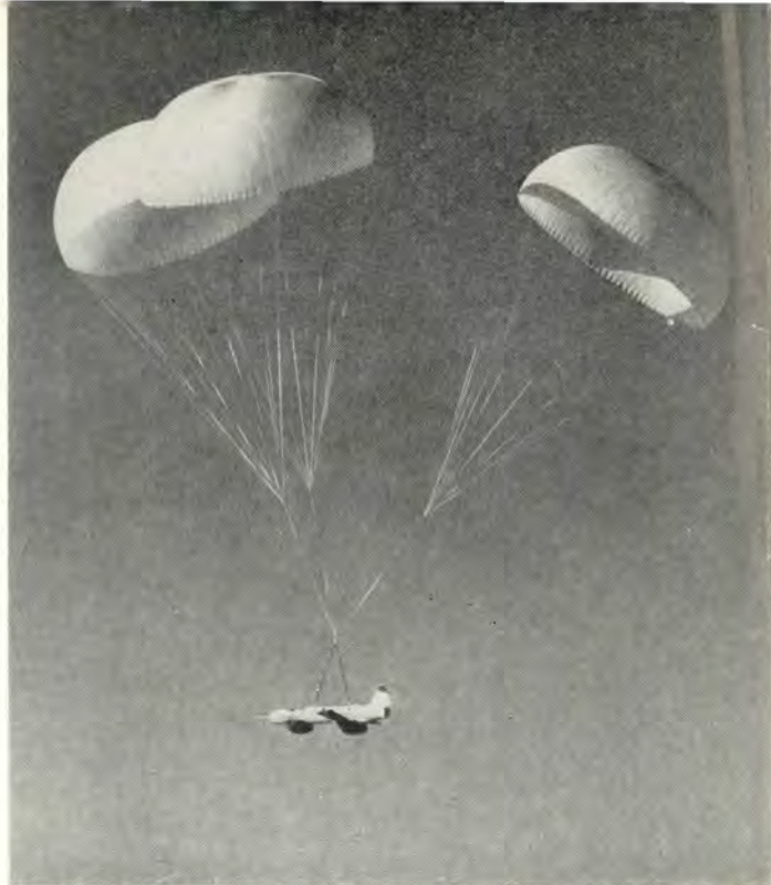
No longer a one-shot weapon, the Martin Matador at $100,000 per copy floats to the ground after flight at the Air Force Missile Development Center in New Mexico. Recovery and re-use will save millions.
