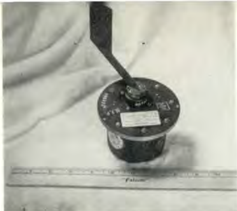
Figure Four. Vane type angle-of-attack detector. Figure five. Probe type angle-of-attack detector.
