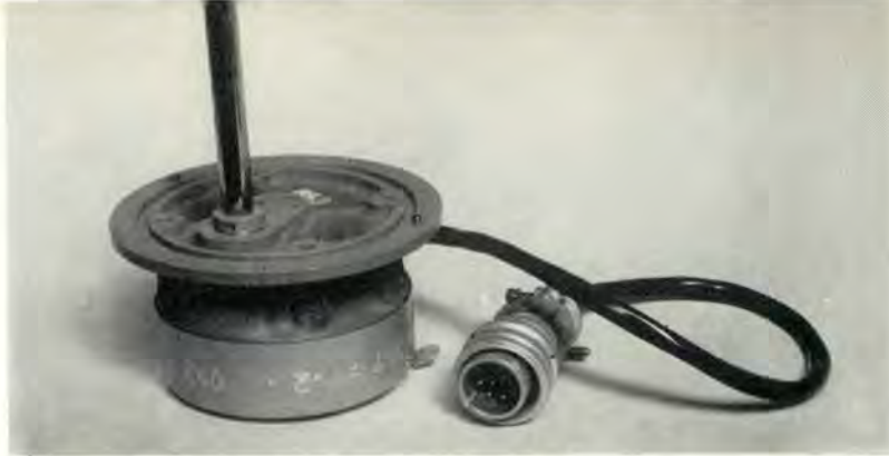
Figure Four. Vane type angle-of-attack detector. Figure five. Probe type angle-of-attack detector.
